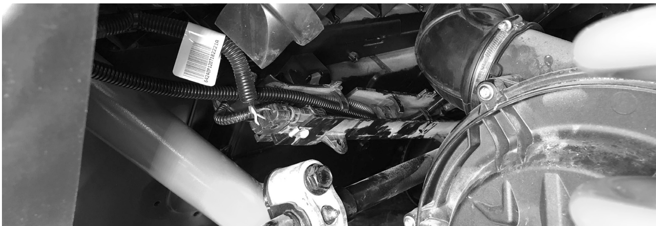
Figure 9b: Shows harness being routed along the left-side cable channel located between the cab and the motor.
