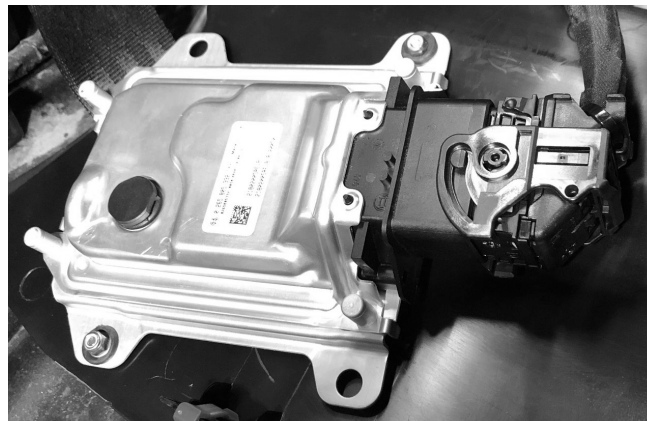
Figure 16b: Locked ECU latch orientation.
