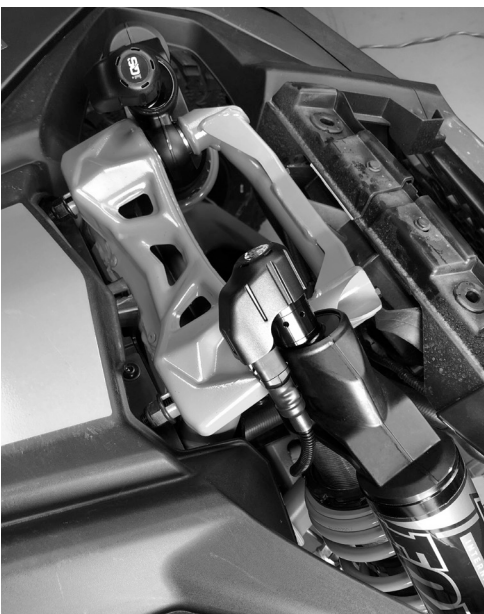
Figure 4c: iQS motor connection facing rearward with leads passing under upper shock mounting bolt.
