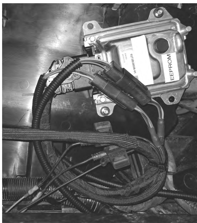
Figure 16c: Shows the ECU installed to the panel and plugged into the main harness with the remaining loose harness loop. Picture taken with driver side console cover removed.
