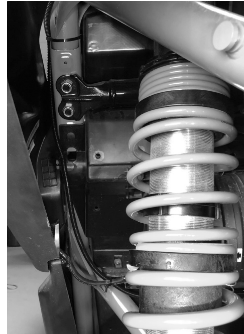
Figure 9a: Shows harness routing along the back of the left-side frame rails before reaching the OEM harness bundle.
