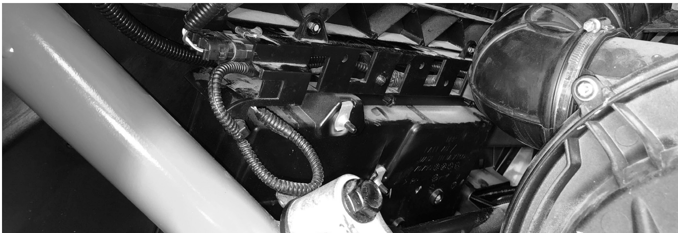
Figure 9c: Shows cable channel installed with the left-side rear shock lead.
